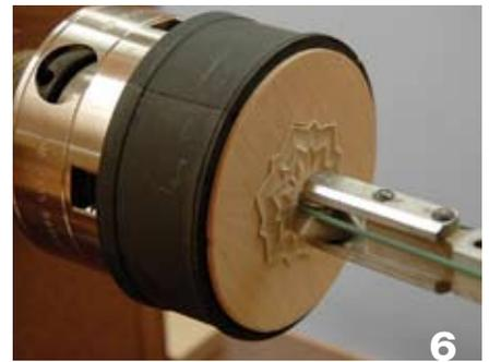
6 Make a series of cuts, adding phasing for interest, across the first face. Reverse the blank and cut the other face to finish the ornamental snowflake.
