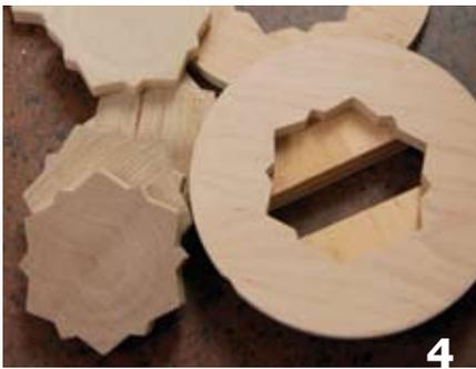
4 Two jig discs and several blanks are ready for rose-engine detailing. Blocks glued to the back of the lower jig provide backing and allow reversing the blanks.
