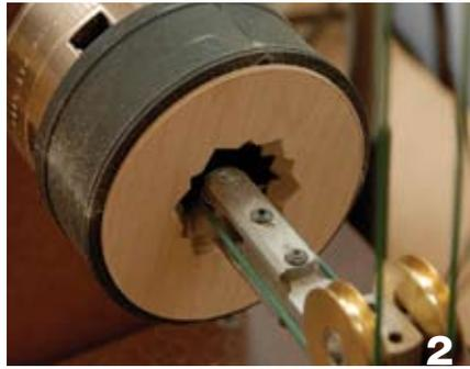
2 Using a horizontal cutting frame and holding the disc in lower jaws, cut the socket all the way through the disc to make the jig.
