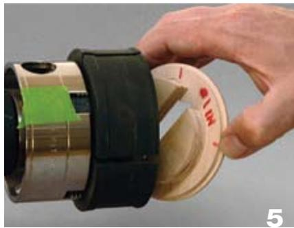
5 Mark the jig on the inside, indicating the left and right edges of the #1 jaw of the chuck. The shoulder and tenon on the disc work as normal.
